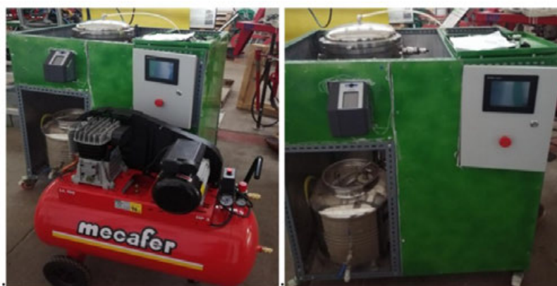
Fig.1 – Extractor biofertilizati/ bioinsecticide concentrați EBB (ADER 25.4.1)
