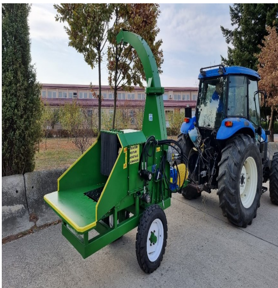
Fig. 1 - Model experimental echipament tocat resturi vegetale TRL-0
