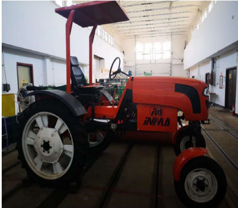
Fig.1 Șasiu sistem de propulsie inteligent (tractor electric)
